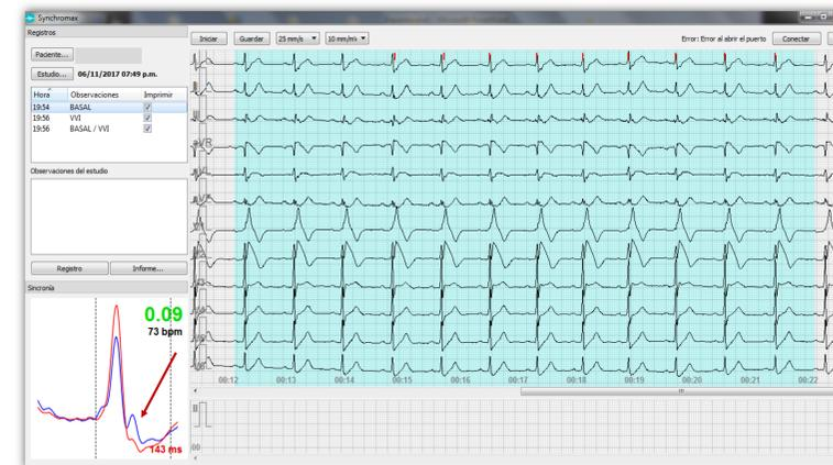
Synchronmax study in a type 1 Brugada pattern patient . Right panel shows 12 leads ECG in real time. In left panel a type 1 curve is observed with 0,09 index. At the end the curves are separated (red arrow). An electric dyssynchrony is present in this area.
